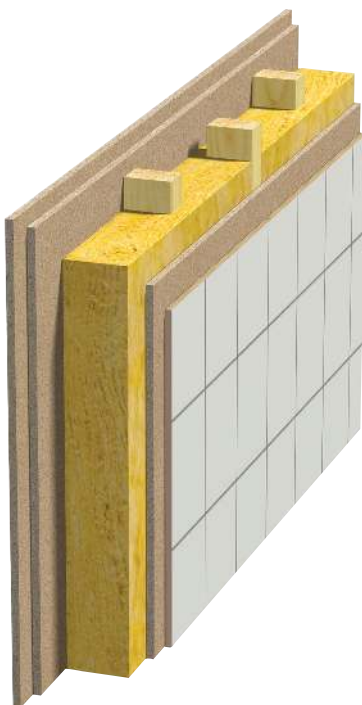
Fig. 3 Internal wall Offset wood studs on wood sill. Double boards.
