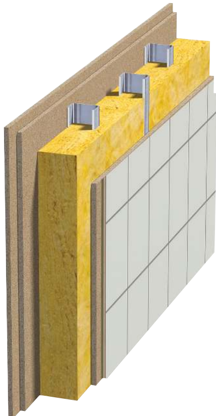
Fig. 6 Internal wall Offset steel studs. Double boards.
