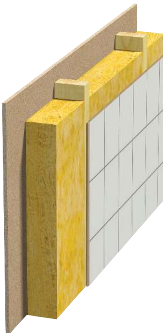
Fig. 1 Internal wall All through wood studs. Single board.
