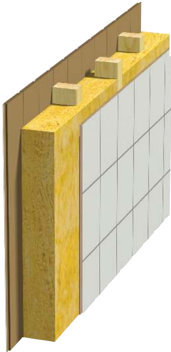
Fig. 2 Internal wall Offset wood studs on wood sill. Single board.
